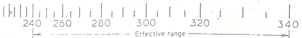
7. Examples of scale markings for vapour pressure thermometers
